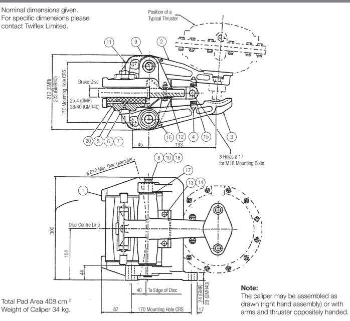
GMR CALIPER ASSEMBLY PART No 6780971 - GMR40 CALIPER ASSEMBLY PART No 6781006
